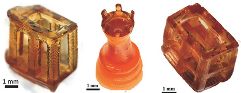
Figure 9. Images of complex, anisotropic 3D structures immediately after printing, using mask-projection micro-stereolithography (MPμSL). The 3D structures contain 85 wt% N-methyl-2-pyrrolidone (NMP) solvent. Reproduced with permission. [139] Copyright 2017, Wiley-VCH.
